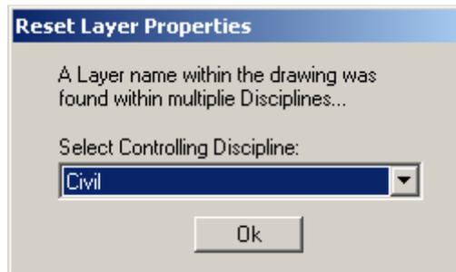
An example use of this feature would be the ability to instantly “screen” layers for one discipline while another discipline “sees” the layers at full weight. Remember that CSM can “reset” Xreferenced layers just as easily as the layers in the current drawing.
