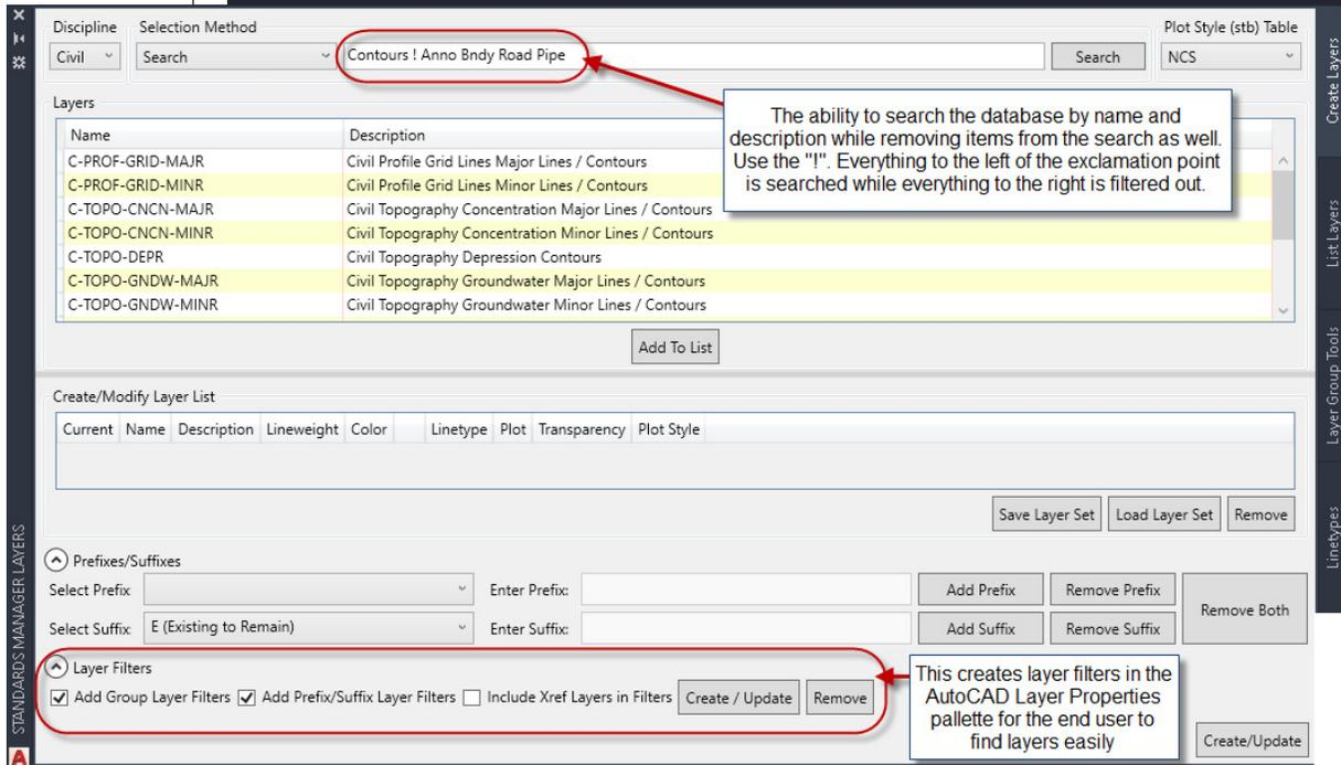
This palette is now modeless and can be docked and manipulated similarly to all AutoCAD palettes. The reworked look is also more streamlined for user efficiency. With the tabs on the palette the user can easily navigate all layer commands at once.
